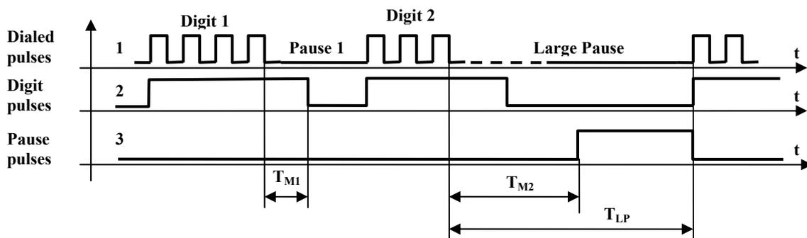
Figure 3. Pulses diagram for period filters from figure 1
