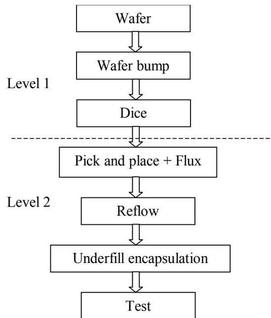
Figure 4. The flip chip process flow
