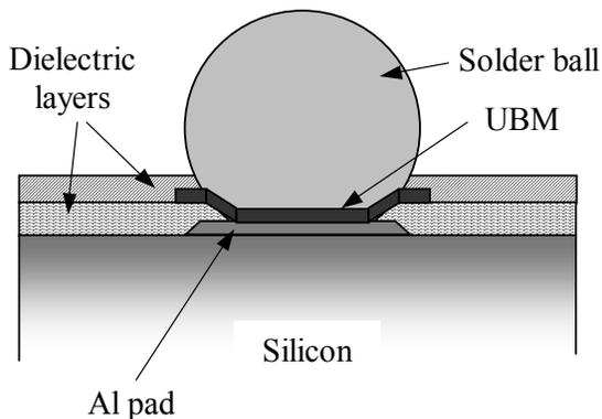
**Figure 5. The solder bumping process**
