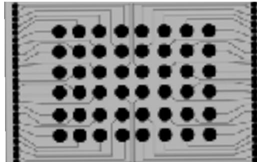
**Figure 6. Redistribution of the peripheral bond pads**
